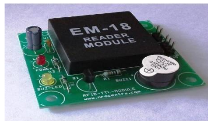
Figure 3: RFID reader module
