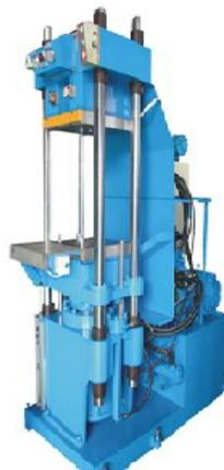
**Figure 3.** Compression moulding machine
