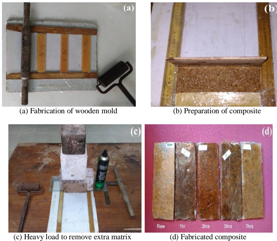
Figure 2.1. Composite Fabrication with different step
