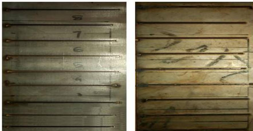
Fig.1 Experimental cuts obtained over (a) 4 mm plate and (b) 12 mm plate thickness
