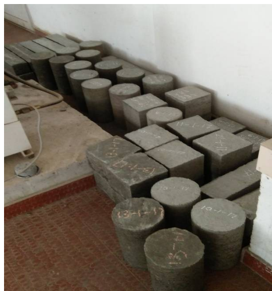
Fig 3 : Air curing of specimens
