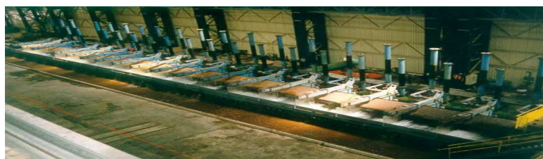
Fig.1 Run out table cooling system
