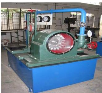
Fig:1 Apparatus of Pelton Wheel Turbine
