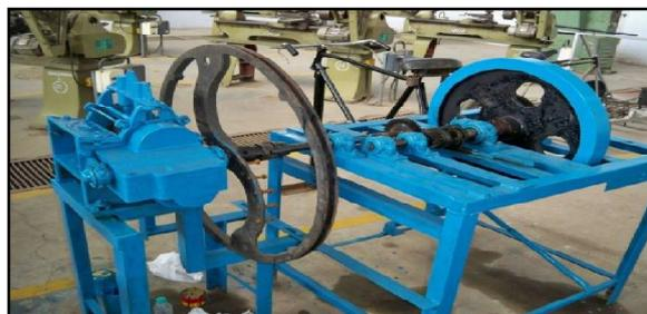
Figure 3: Establishing empirical relationship for chaff cutter energized by human powered flywheel motor
