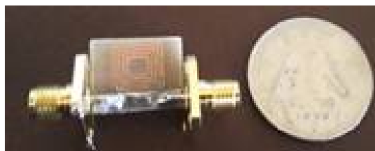
Fig 11. Photograph of Fabricated filter with Spiral Resonator Stub on Microstrip Transmission line.
