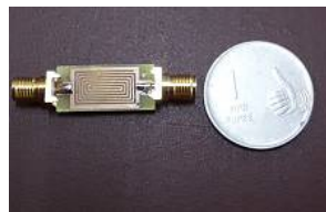
Fig 16. Photograph of Fabricated filter with Spiral Resonator embedded in Microstrip Transmission line.
