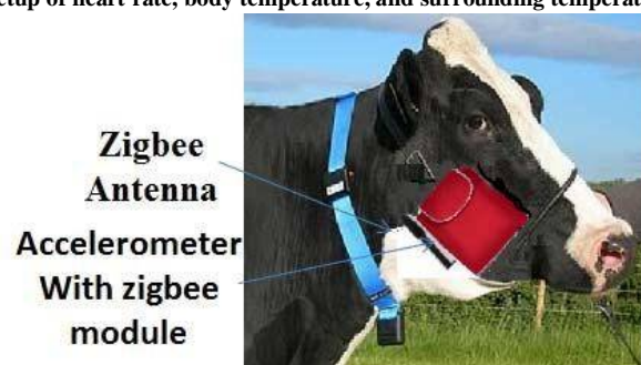
Fig. Experimental setup of rumination sensor module.
