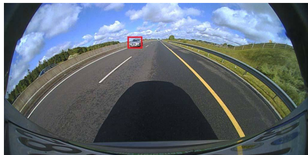
Fig. 4. View from fisheye camera mounted at the rear of a BMW X5 with AdaBoost detection of an approaching vehicle encapsulated in the red bounding box
