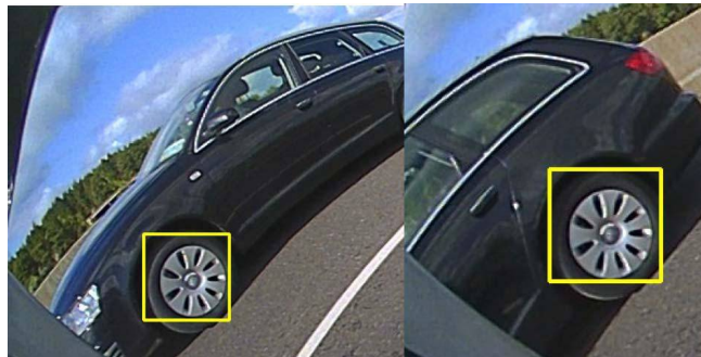
Fig. 6. Detection of front and rear wheels at edge of the image using the Hough Circle Transform.
