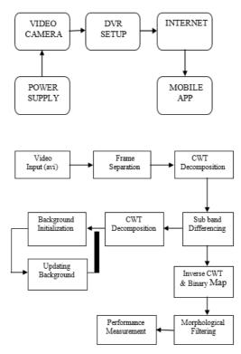
An input video file in avi format is given to the system. The video file is parsed into a sequence of images called frames. The frames are then decomposed using composite wavelet transform and then subband differencing is performed. The frames are decomposed into foreground and background which are mapped after the subband differencing process and inverse composite wavelet transform is carried out. Morphological
