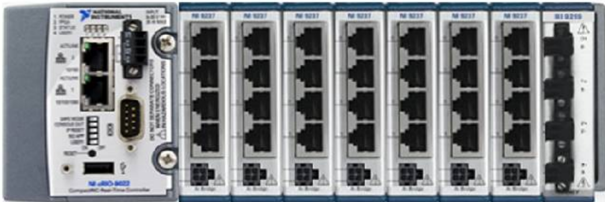
CompactRIO data acquisition system with NI-9237 modules (wired).
