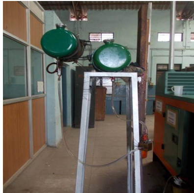
Fig.2 shows the fuel tanks.
