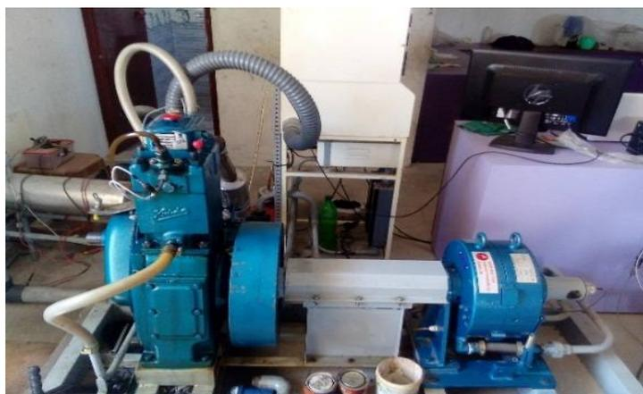
Figure: Kirloskar TV1 Engine Experimental setup
