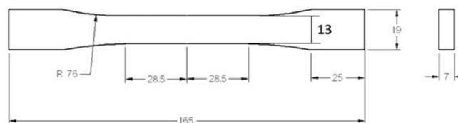
**Figure (a): Tensile Test Sample as per ASTM D638 (Type I)**
