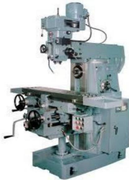
**Fig 1: Vertical Milling Machine**
