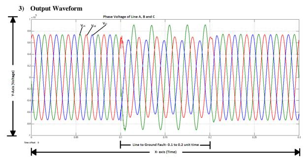
The transmission line model system was simulated to identify the type of fault on the affected phase. The system was designed with a means of observing all the phases on the transmission line on one platform, using the scope in MATLAB/SIMULINK. In a double phase fault, two of the signals with faults indicated some deviations from the expected wave form. When the type of the fault had been established, fault data, which can be referred to as signal from
