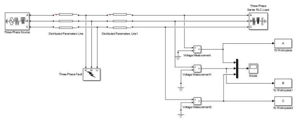
We have one three phase source and the transmission line is given. We created fault in transmission line. We measure the magnitude of the voltage in healthy condition & after faulty condition.
