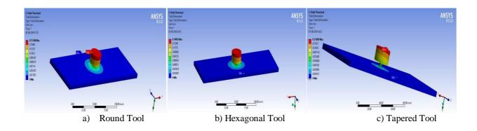
On detailed observation, we get to know the stress values for four different types of tools. On the basis of the stress values thus obtained, we derive conclusion and can decide the better tool for conduction of friction stir welding.
