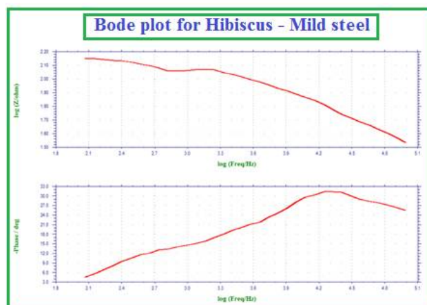
Fig 9: AC impedance spectra (Bode plot) of Mild steel immersed in Hibiscus Extract
