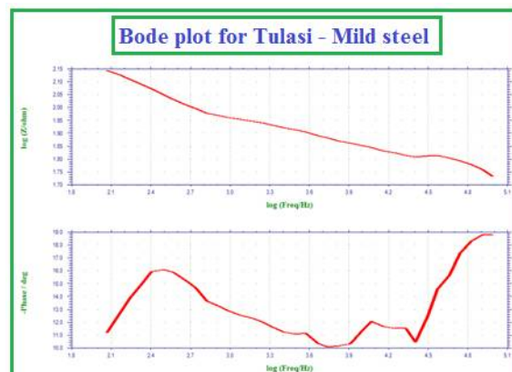
Fig 7: AC impedance spectra (Bode plot) of Mild steel immersed in Tulasi Extract
