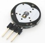
The sensor shines a light lobe (a small very bright LED) through the ear and measures the light that gets transmitted to the <u>Light Dependent Resistor</u>. The amplified signal gets inverted and filtered, in the Circuit. In order to calculate the heart rate based on the blood flow to the fingertip, a heart-rate sensor is assembled with the help of <u>LM358</u> <u>OP-AMP</u> for monitoring the heartbeat pulses.
