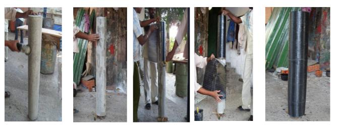
fig .3 shows Surface Preparation and cleaning of the specimen
