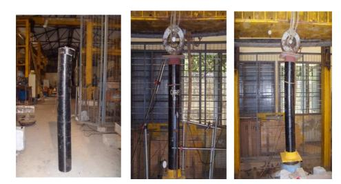
Fig. 5 Testing Setup CFRP Wrapped Specimen
