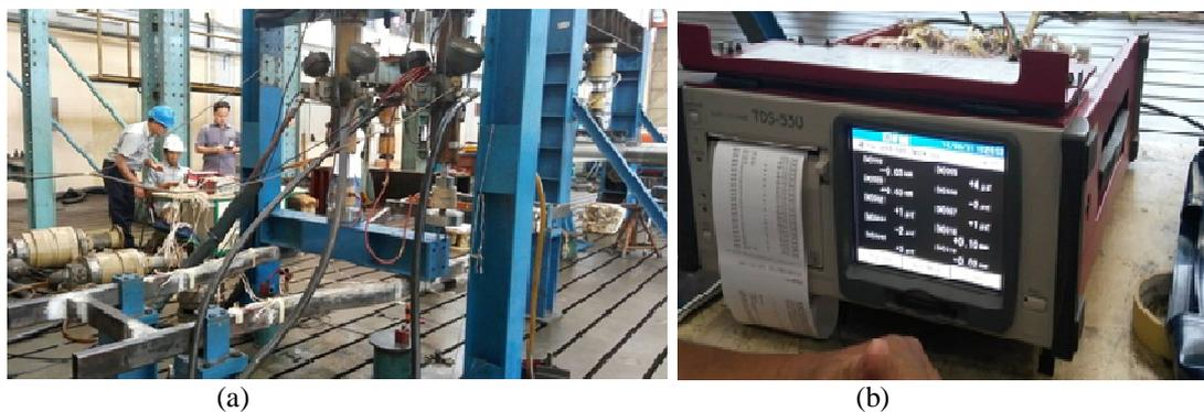
Figure 11. (a) Static Test Prototype Chassis, (b) Data Record Equipment
