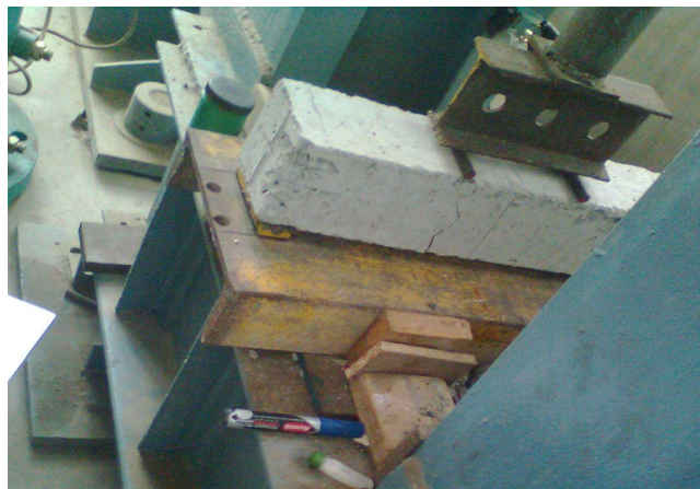
Fig.2: Specimen under flexural test
