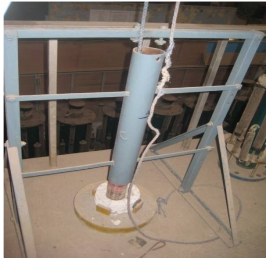
Fig.4 : Specimen under impact load
