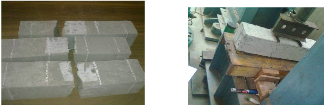
Fig. 20: Failure pattern of control and FRC
