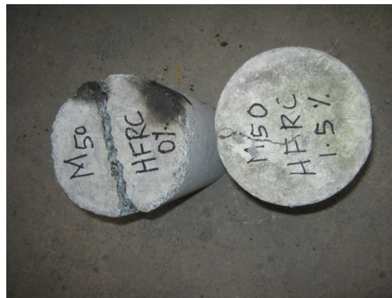
Fig.13: The failure patterns of control and FRC
