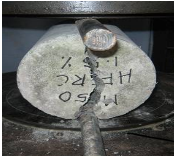
Fig.3: Specimen in compression testing machine
