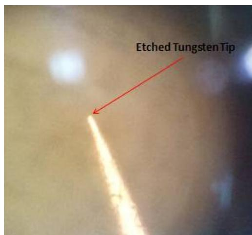
Fig 7: Optical image of Tungsten tip (5X)
