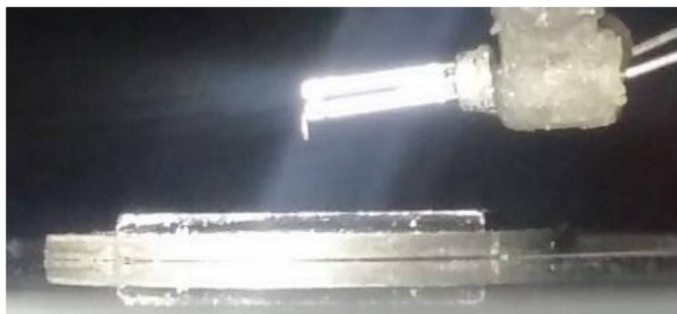
Fig 1: QTF with Tungsten tip attached
