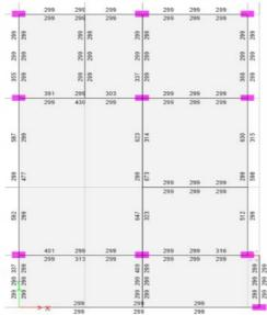
Fig 1:Reinforcement details of model 1 ground floor
