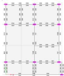
Fig 2: Reinforcement details of model 2 ground floor
