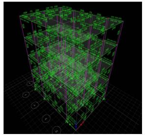
Fig 4:Reinforcement details of Model 2 in 3D view
