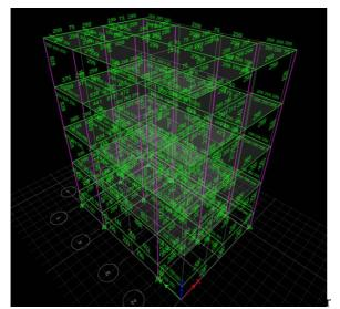
Fig 3:Reinforcement details of Model 1 in 3D view
