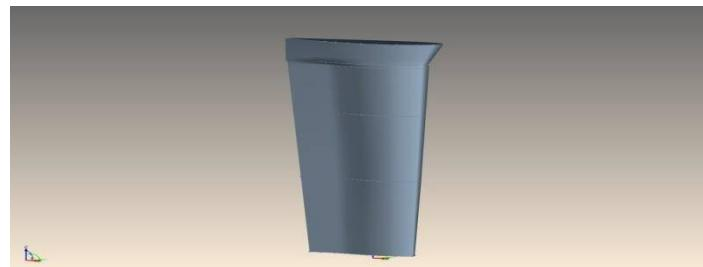
Figure 9. Schilling rudder geometry
