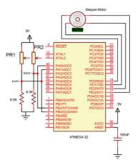
Microcontroller requires a 5 In the solar tracker prototype, it is desired that output voltage at junction point will increase as the light intensity increases and so the photo resistor is placed at the top position in series connection with resistor.
