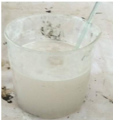
Fig 2: Mixing of solutions ( $\text{NaOH}$ &Water)
