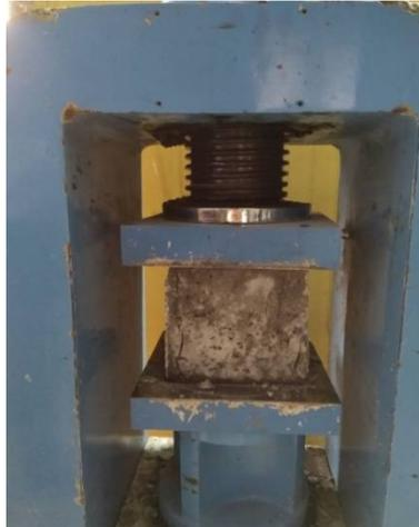
Fig.3. Testing of cube in compression testing machine
