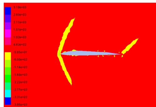
Fig. 25 Velocity derivative plot of  $40^\circ$  Swept wing at  $0^\circ$  AOA Turbulence intensity of 15% and at 1.2Mach
