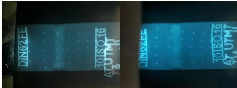
Figure 2 Xray radiography of welded specimens
