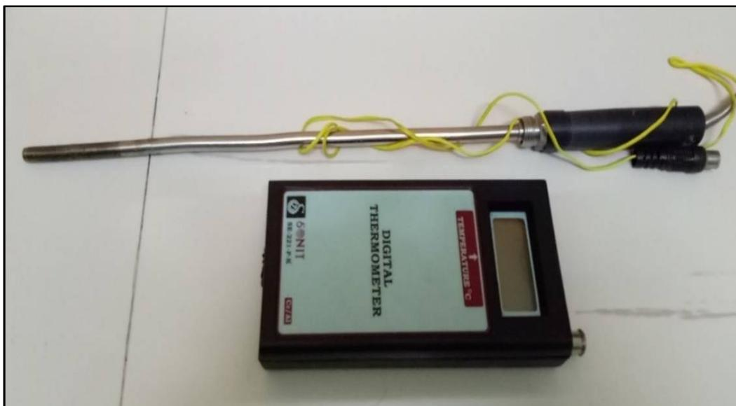
Figure 16Digital thermometer
