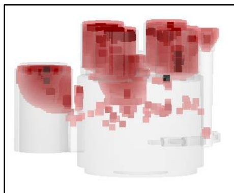
Fig: 3 Shrinkage Defect predictions by simulation
