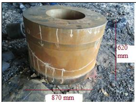
Fig: 1: Shrinkage occurs at the center of casting
