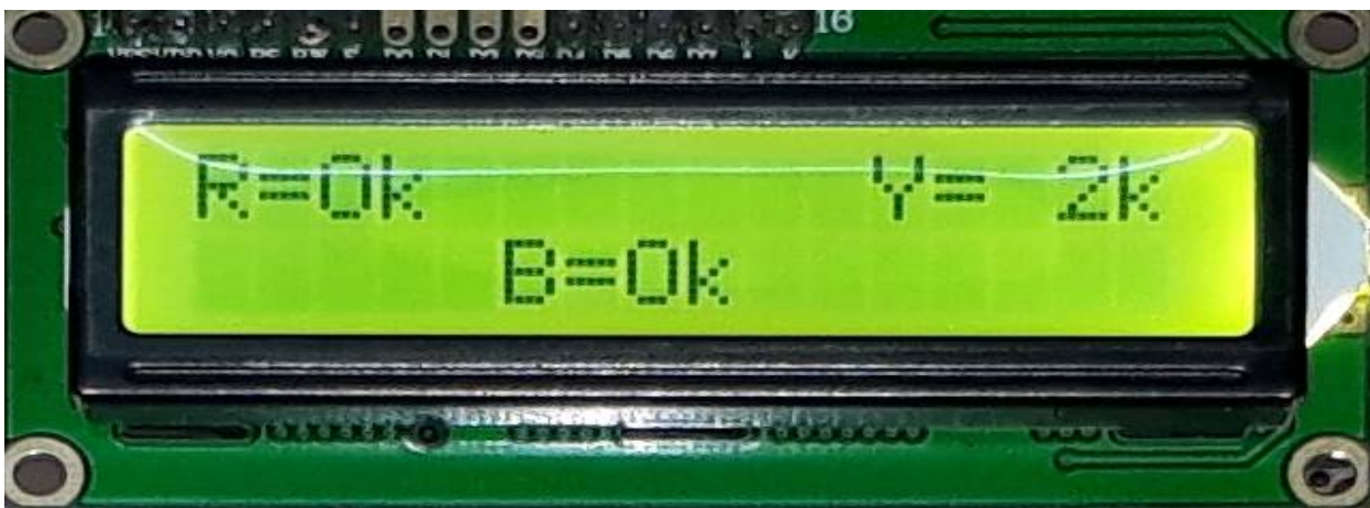
Fig.5(a): LCD View for Fault at 2 Km
