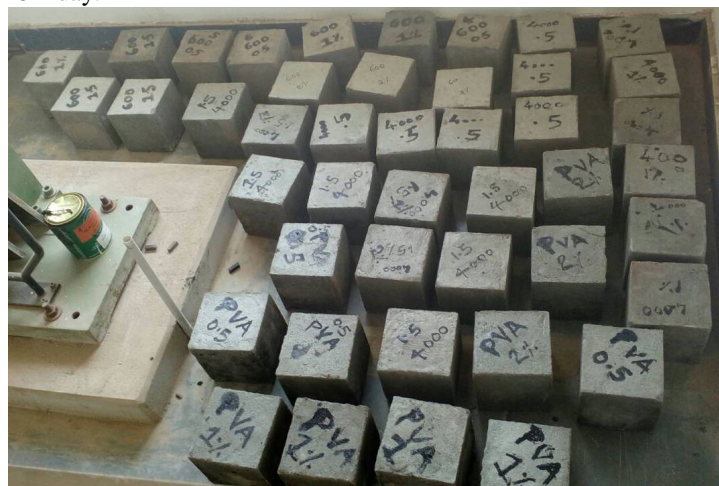
Fig 2: Specimens kept for curing in ambient temperature.
