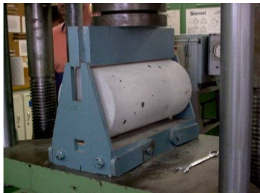
Fig.3: Split Tensile Testing Machine
