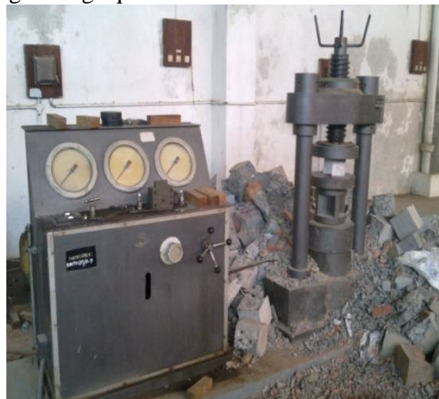
Fig.2: Compressive Strength Testing Machine
