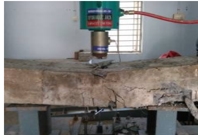
Fig: 4 Initial crack formation
