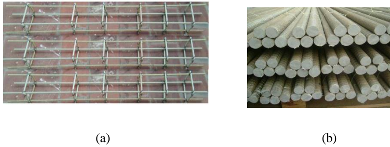
Fig. 1. Preparation of specimen (a) reinforcement steel (b) GFRP
