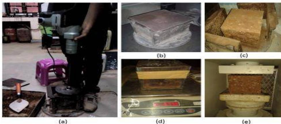
Fig. 3 Sequences involved in preparation and testing of UCS of cube specimens (a) Compaction of materials in a cube mould using a vibratory hammer, (b) cube mould covered with a metal plate (160 mm x 160 mm x 3 mm), (c) removal of specimen from the mould after 24 hours (d) weight measurement of cube specimen inside a properly sealed curing tin (160 mm x 160 mm x 155 mm), (e) Unconfined compression test of specimen (after 7 days) using a Compression testing machine
