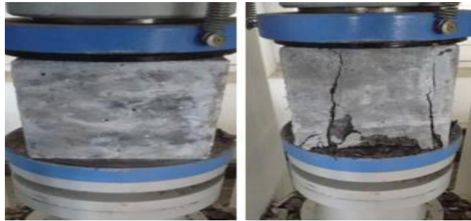
Fig3: Compression testing of cube
