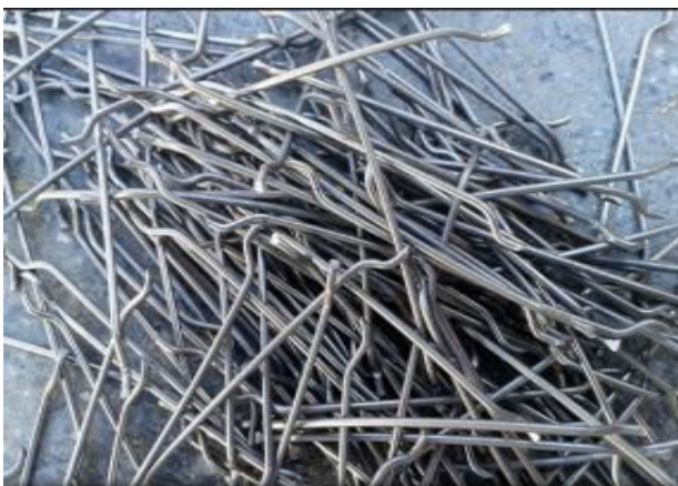
Fig1: Hooked-end steel fibers
