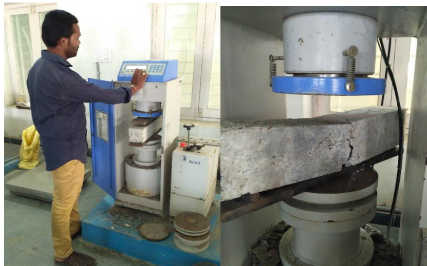
Fig4: Flexural testing of beam
