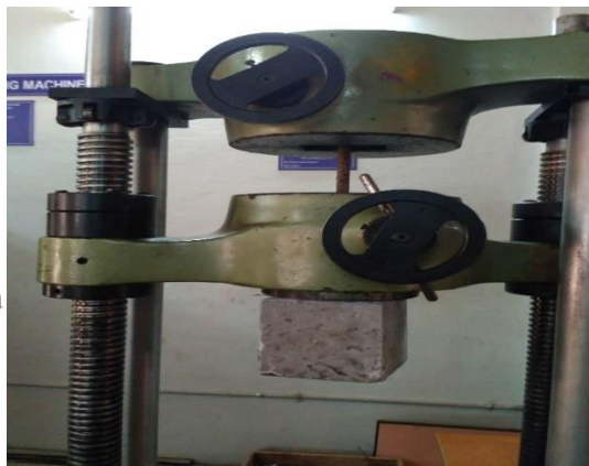
pull out test under progress
