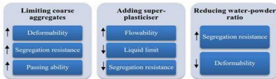
Figure 1: Mechanisms of achieving self-compactability [3]
