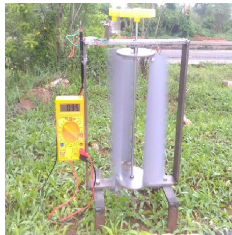
Figure 6 Fabricated model of small VAWT Figure 7 Fabricated model of small VAWT in highway median
