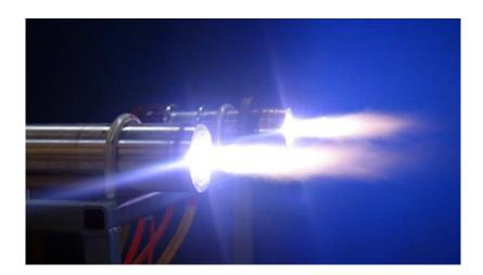
The plasma torches used in these facilities are custom-built. The amount of energy they consume, the lifespan of the electrodes it uses, the gas used for ionization (most torches just use ordinary air), the downtime it takes to replace an offline torch and the size of the plasma field it generates all depend on the specific manufacturer. Plasma torches are water-cooled.
