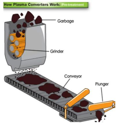
Although a plasma torch can break down waste without any special pre-treatment, most plasma facilities employ some sort of pre-treatment process to make the entire system more efficient. Some designs use grinders or
