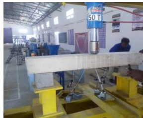
Fig 8: Beam setup on loading frame
