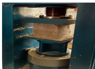
Fig 3 Compression test of cubes
