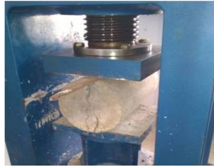
Fig 6 Split tensile test of cylinder
