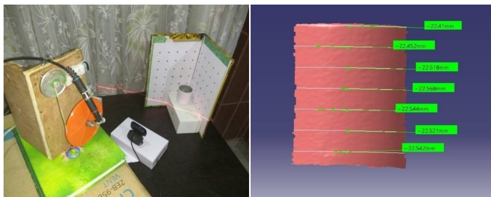
Fig. 4 (a) Shows the experimental set up of Semi Automatic Laser Light Scanning (b) Shows the scanning results obtained by Semi Automatic Laser Light Scanning
