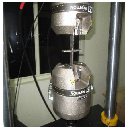
Fig 3 : Specimen placed in Fatigue testing Machine
