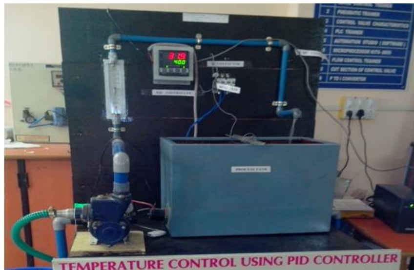
Fig 1: Temperature Control System
