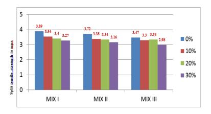
The above Figure shows the split tensile strength of 28 days result observed for 30% of RCA and different % of fly ash in various mix proportion of concrete. The above result 28 days result observed the optimum percentage of split tensile strength. This result higher than the control mix I days result.
