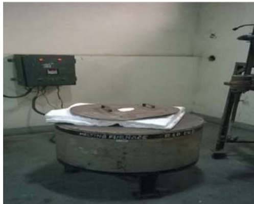
Figure 1: Electric Arc Furnace
