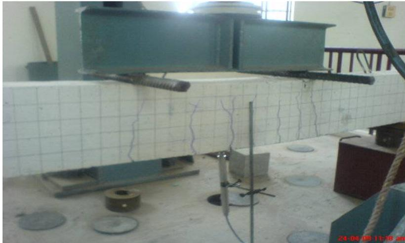
**Fig 7 Testing of Ordinary RCC Beam**
