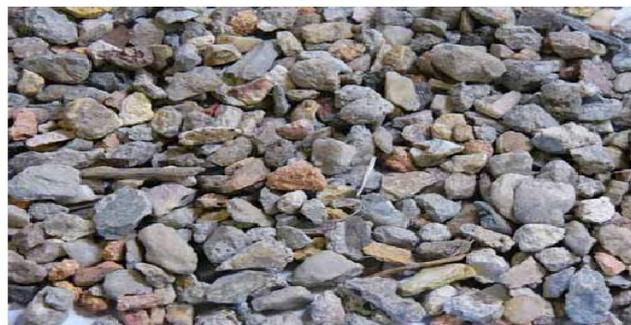
Fig 1. Recycled Coarse Aggregate
