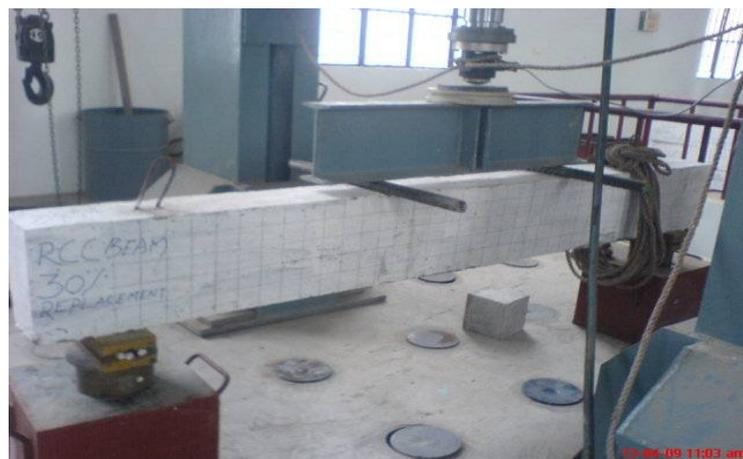
Fig .2 Experimental Set-up of Beam with Loading Frame
